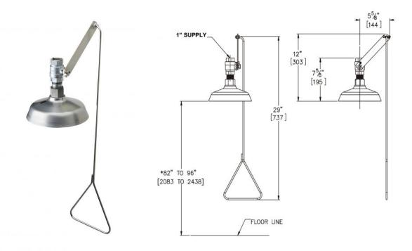
Model S2100 is our vertical ceiling mounted safety shower with stainless steel head. Supplied with stainless steel shower head, stainless steel pull handle and 1" chrome plated brass stay open ball valve.
